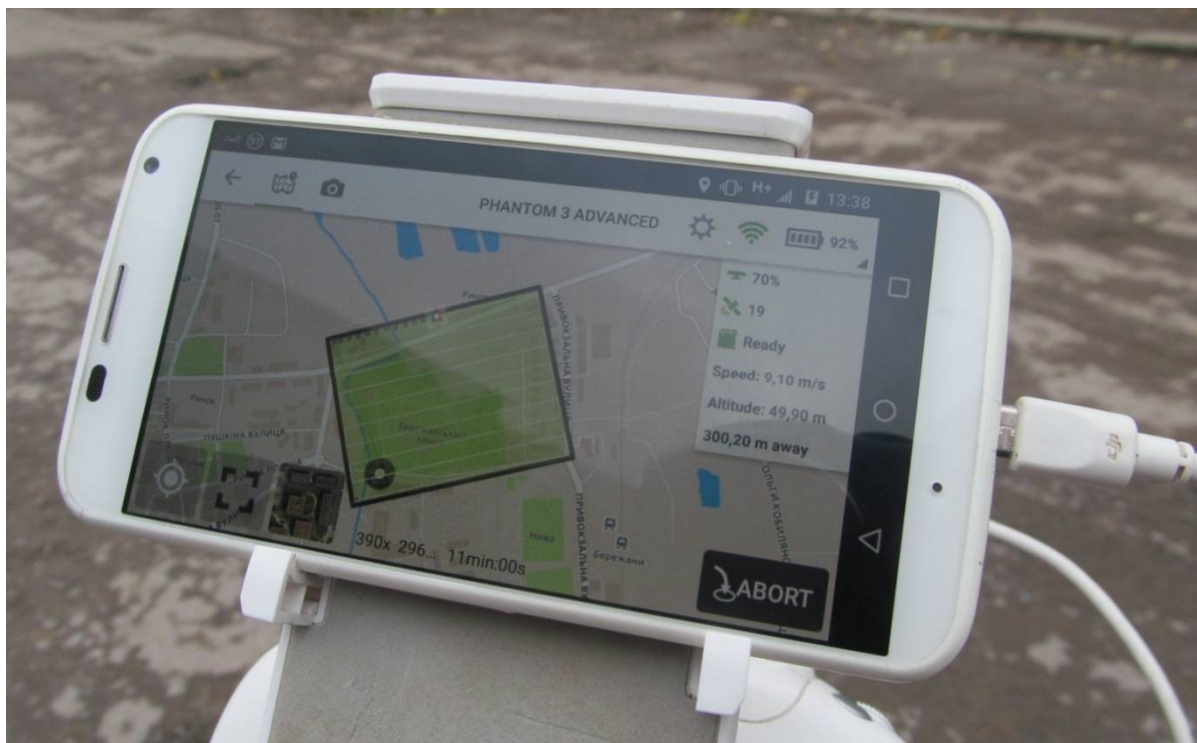
Fig. 1. A planned route of a drone in order to perform Berezhany castle park surveying
